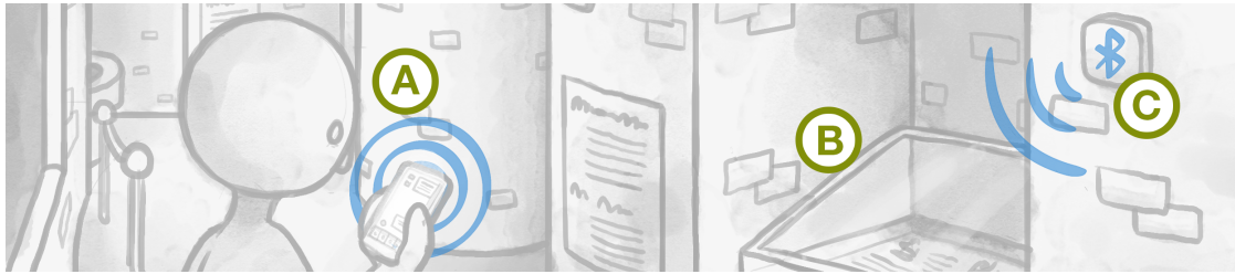
Figure 6.1: Museum setting showing the visitor using the mobile application with visualization (a), the physical object in the museum (b), and Bluetooth beacons at exhibits telling the app where the user is located (c). Illustration by M. Boucher.
