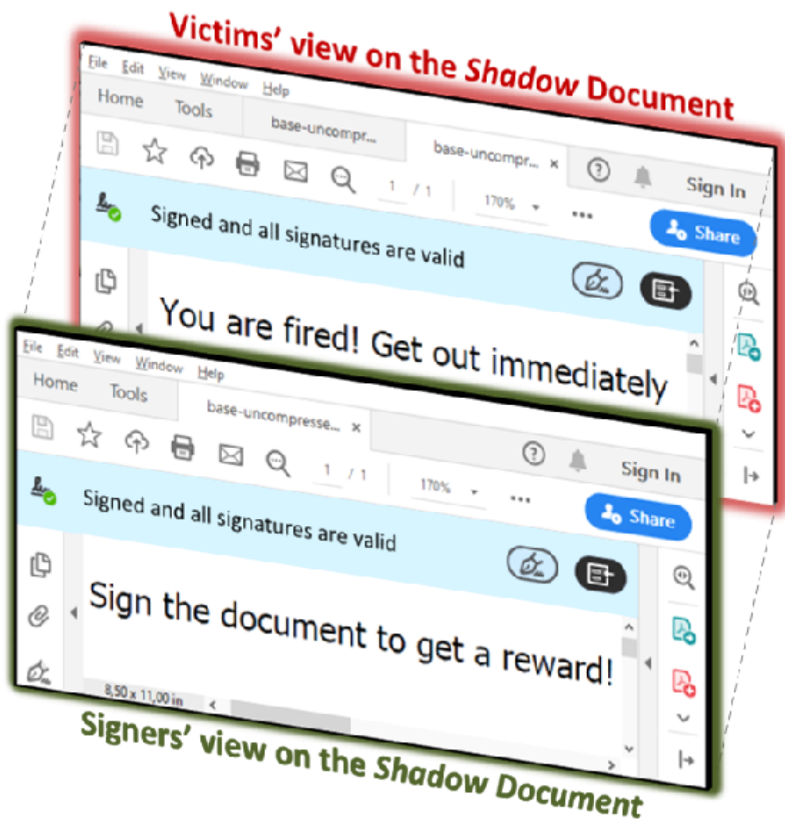
Figure 3.1.: The example shows, that the person that digitally signs the document has a different view [3] of the document. After the digital signature process, the attackers swap the prepared content without invalidating the digital signature.
