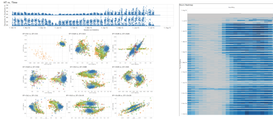
Figure 6: Bridge vibrations: Linked views depict seasonal patterns (top) and daily trends (right) of bridge transits as well as correlations between dimensions of the resulting vibrations (bottom).
