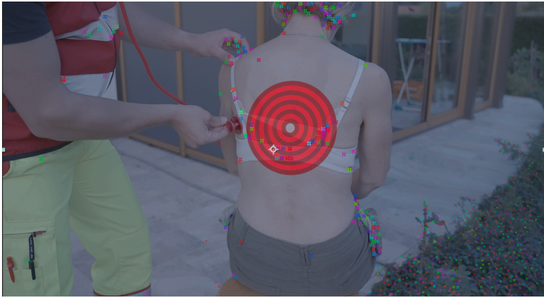
Figure 41: 3D Camera-Tracking points with a red target circle
