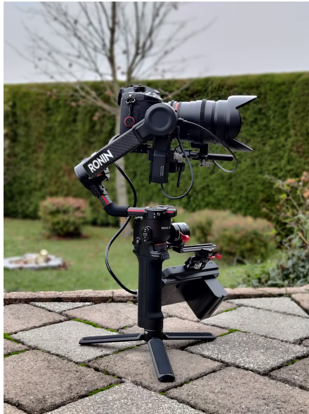
Figure 39: Ronin RS2 gimbal with mounted camera
